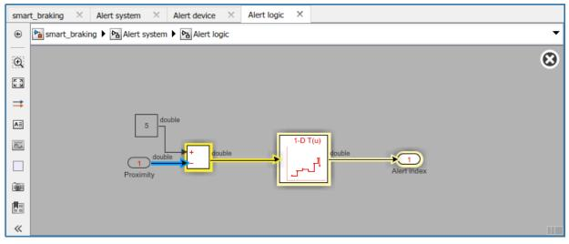
**5** To find the source of the discretization, keep pressing the left arrow and note the colors of port names that reflect the sample time.
