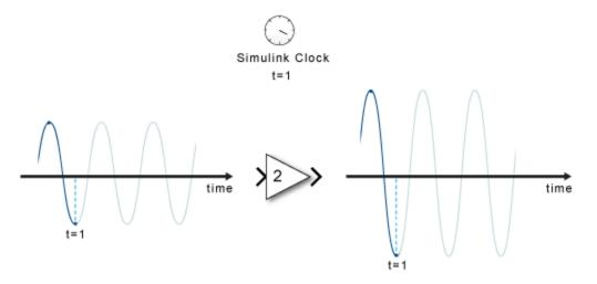
At each time step, each block computes its outputs from its inputs. Once all the signals in a diagram are computed at a given time step, Simulink determines the next time step (based on the model configuration and numerical solver algorithms) and advances the simulation clock. Then each block computes their output for this new time step.
