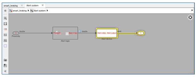
4 Keep tracing the signal to its source until you reach the Alert logic subsystem. You see that the Subtract block has two inputs. Choose the signal path from the Inport by pressing the down arrow key.
