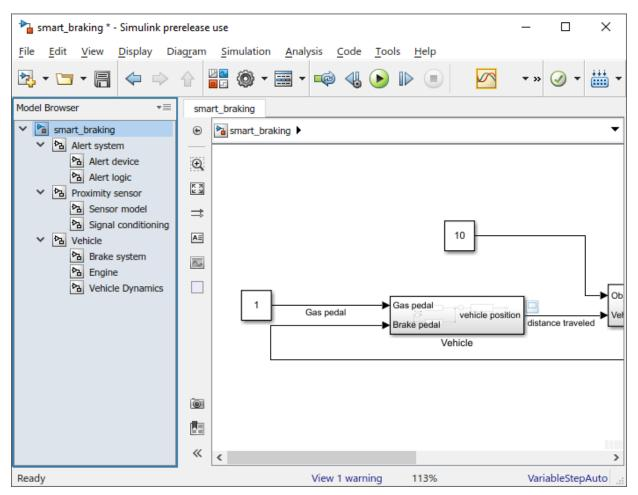
The Model Browser shows that all subsystems you view at the top level also have subsystems of their own. Click > icons to see the subsystems. You can navigate through the hierarchy in the Model Browser. For example, click the Sensor model subsystem:
