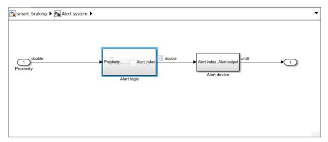
The labels in this subsystem suggests that data type change occurs in the Alert device subsystem, double-click to investigate:
