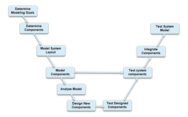
The workflow in this tutorial focuses on fundamental Simulink tasks as they relate to Model-Based Design.
