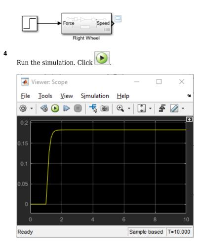
The simulation result exhibits the general expected behavior. There is no motion until force is applied at step time. When force is applied, the speed starts increasing and then settles at a constant when the applied force and the drag force reach an equilibrium. Besides validation, this simulation also gives information on the maximum speed of the wheel with the given force.
