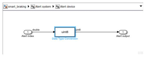
This shows that the Alert device component converts the alert index signal from a double to an integer. You can set the data type at sources, or use a Data Type Conversion block from the Signal Attributes library. The double data type, the default, provides the best numerical precision and is supported in all blocks. It also uses the most memory and computing power. Other numerical data types serve to model typical embedded systems where memory and computing power are limited.
