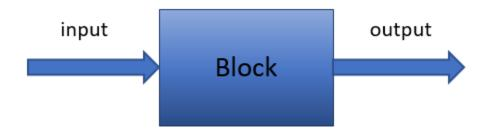
A block can represent a physical component, a small system, or a function; an input/ output relationship fully characterizes the block. Consider these examples:
