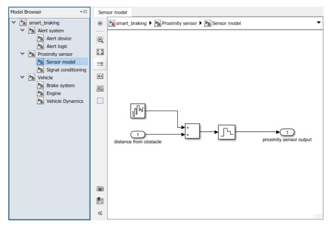
Observe that the subsystem is highlighted in the Model Browser. The address bar also shows which subsystem you are viewing. To open the subsystem in a separate window instead, right-click the subsystem name and select **Open In New Window**.
