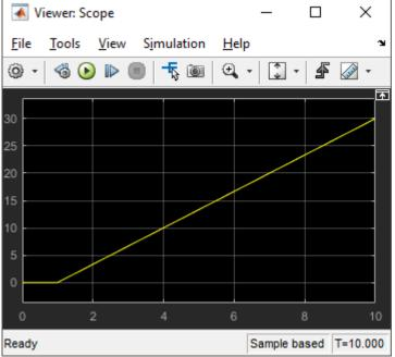
This simulation shows that the angle increases steadily when the wheels are turning with the same speed in opposite directions. You can make some model improvements to make it easier to interpret the angle output, for example:
