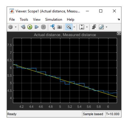
From the plot, you can see that the measurement can deviate from the actual value by as much as 0.3 m. This information becomes useful when designing a safety feature, for example, a collision warning.
