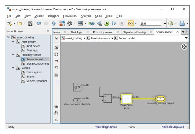
You find that the Zero-Order Hold block in the Sensor model subsystem does the conversion from continuous to discrete.
