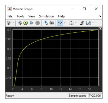
At time 3, the position of the robot is at about 0.55 m, and when the simulation ends, it is less than 0.71 m. It is safe to say that the robot travels less than 0.16 m after the power is cut.
