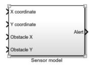
2 Construct the distance measurement. In the sensor model block, use Subtract, Math Function with magnitude^2 function, Sum, and Sqrt blocks as shown. Note the reordering of the input ports.
