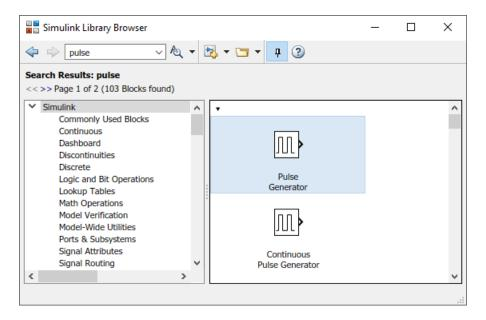
Get detailed information about a block. Right-click a block, and then select **Help for the Pulse Generator block**. The Help browser opens with the reference page for the block.
