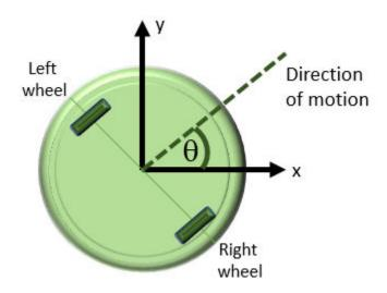
Each type of motion starts from a resting state, that is, both rotational and linear speeds are zero. With these assumptions, linear and rotational motion components can be modeled separately for this introductory tutorial.
