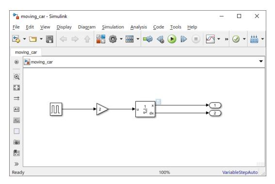
Simulating this model integrates a brief pulse twice to get a ramp. The results display in a Scope window. The input pulse represents a press of the gas pedal -1 when the pedal is pressed and 0 when it is not. The output ramp is the increasing distance from the starting point.
