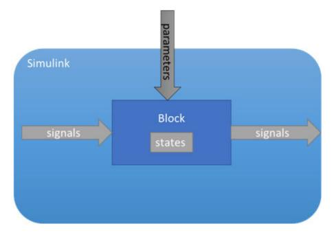
At each time step, Simulink computes new values for signals and states. By contrast, you specify parameters when you build the model and can occasionally change them while simulation is running.
